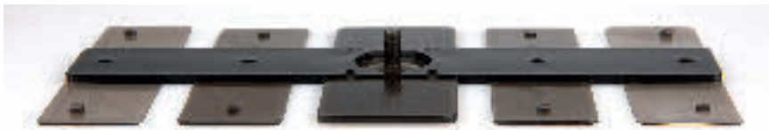
Fig. 4. Stepped panel with four different wall thicknesses. The center web is 3 mm thick. The side arms have wall thicknesses of 2, 1 and 0.5 mm, with the thinnest regions located at the end of the flow path © Engel
