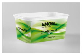
The food containers have a wall thickness of 0.4 mm including the label. At the trade fair, an e-speed 420/90 injection moulding machine with integrated IML will be used to produce ready-to-use margarine tubs by means of a fully automated injection compression process. (Image: ENGEL)
