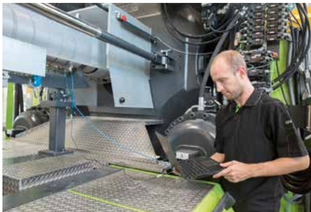
Fig. 3. The data collection – at Schöfer in this case, on an Engel duo16050/1700 with a 135 mm screw – only takes few minutes. The measurement results are evaluated automatically (© Engel)
