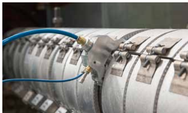
Fig. 1. The new measurement system can be easily installed externally on the melt cylinder, as here at Praher Plastics Austria on a tiebarless machine with 5000 kN clamping force (© Engel)
