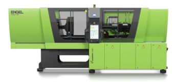
Process integration is key to reducing production costs. The heated thermoplastic sheet is formed in the injection moulding machine and immediately overmoulded to create the reinforcing and functional elements. (Picture: ENGEL)
