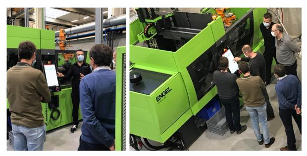
PlastIQ and ENGEL Benelux have created new training capacities at the Kortrijk and Genk sites. The two new machines are each equipped with an ENGEL viper linear robot and intelligent assistance systems from ENGEL's inject 4.0 programme.
