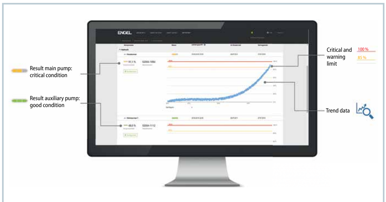
Fig. 3. The condition of the hydraulic oil and the pumps (shown in the screenshot) is clearly displayed on the e-connect customer portal. The system can automatically send status messages and warning messages (© Engel)
