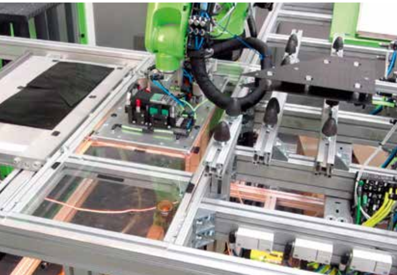
A video-optical measuring system has been integrated to determine the actual position of the tapes on the laying head of the experimental setup (© Engel)
