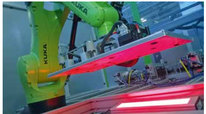
Fig. 6. Investigating direct and indirect illumination during imaging: Illumination is a key factor for exact edge detection (© Engel)
