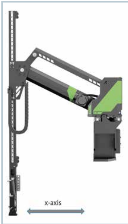
Fig. 2. Instead of a conventional x-axis, type e-pic robots have a rotational axis, which also ensures that the system requires minimum space (© Engel)
