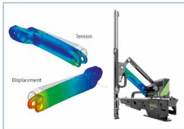
Fig. 3. The rotational axis was designed with an assembled profile of carbon tapes and a stub of die-cast aluminum for connecting to the servo motor (© Engel)
