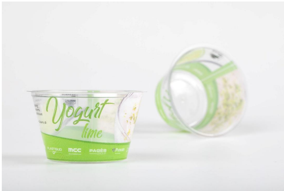
Image 1: Recyclable, lightweight and future-proof: These thin-wall PET yoghurt cups with 30% bottle-grade rPET already meet the 2030 requirements of the PPWR and demonstrate how sustainability and product quality go hand in hand in injection moulding.
