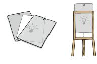
Draw or print a design of your choice on a A3 sheet (plain paper) to highlight it. Simply slide your work between the two diffusers (opaque diffuser at the back) before mounting it on the lamp.
