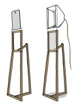
Slide the diffusers into the grooves of the frame. Now slide the shade onto the frame until it rests on the stopper at the back.
