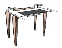
Slide the tray from the front to the bottom as shown in the diagram.
