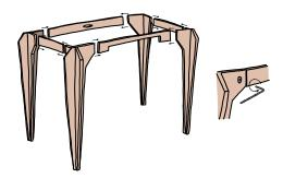
Assemble the leg parts together using the hex key (supplied) as shown in the diagram.
