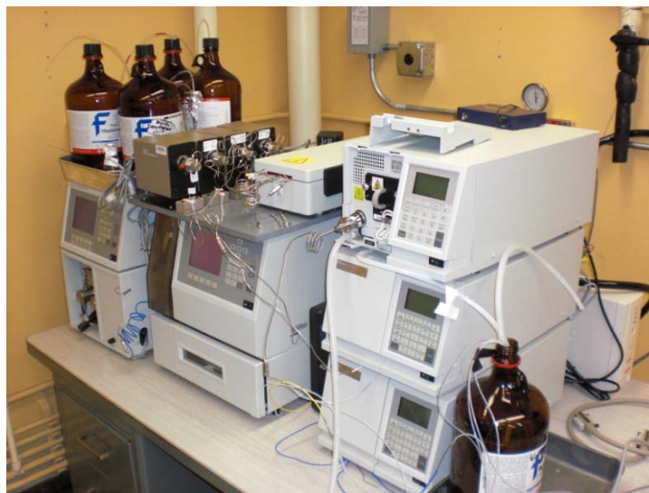
Figure 1. Photo. The automated SAR-AD apparatus setup at WRI.
