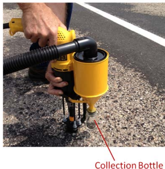
Figure 3. Photo. Micro-sampling with a venturi collector system.
