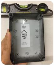
3) Drill the correct size hole in the bottom of the EO Mini base to take the cable gland. Note that cable entry must be from below to ensure weathertightness of the enclosure. Use
