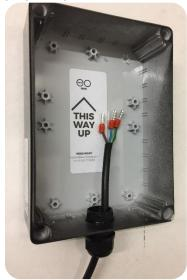
8) Connect the power cable to the front plate of the EO Mini.
