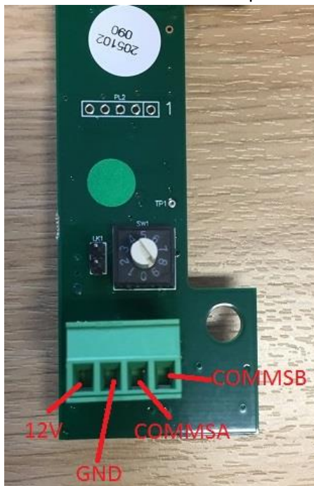
Figure 5 - Wiring connection for the EO Mini
