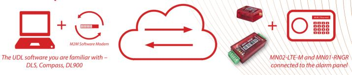
MN02-LTE-M supports remote UDL via add-on MN01-RNGR module connected to the RING/TIP terminals for select panels (DSC, Honeywell and GE NX series)
