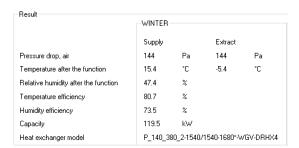
In this case we decrease the pressure drop from 188 Pa to 144Pa and we increase the efficiency from 78,3% to 80,7% by selecting the ECO version of the heat exchanger.
