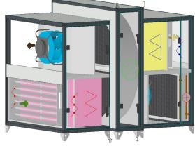
By selecting the ECO version of the heat exchanger the system will insert the heat exchanger from one unit size larger. In the above Geniox 16 the rotary heat exchanger section from a Geniox 18 is inserted.
