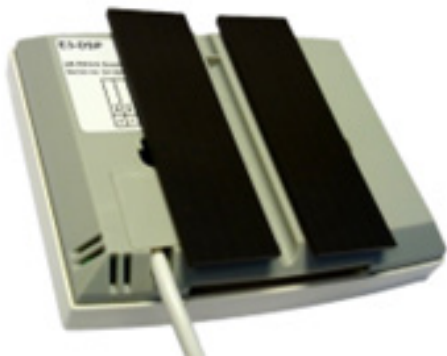
Figure 2. Bottom exit of the electrical connection cable.
