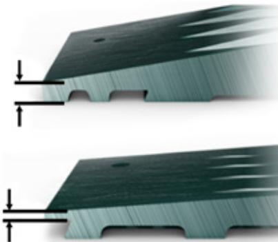
Jaws with locking wedges in the back can wear to a thickness of 60-65 mm until they must be changed.
