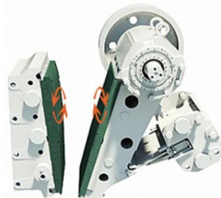
This procedure allows for good work hardening of the manganese jaw dies, and helps maintain the best nip angle for maximum throughput.
