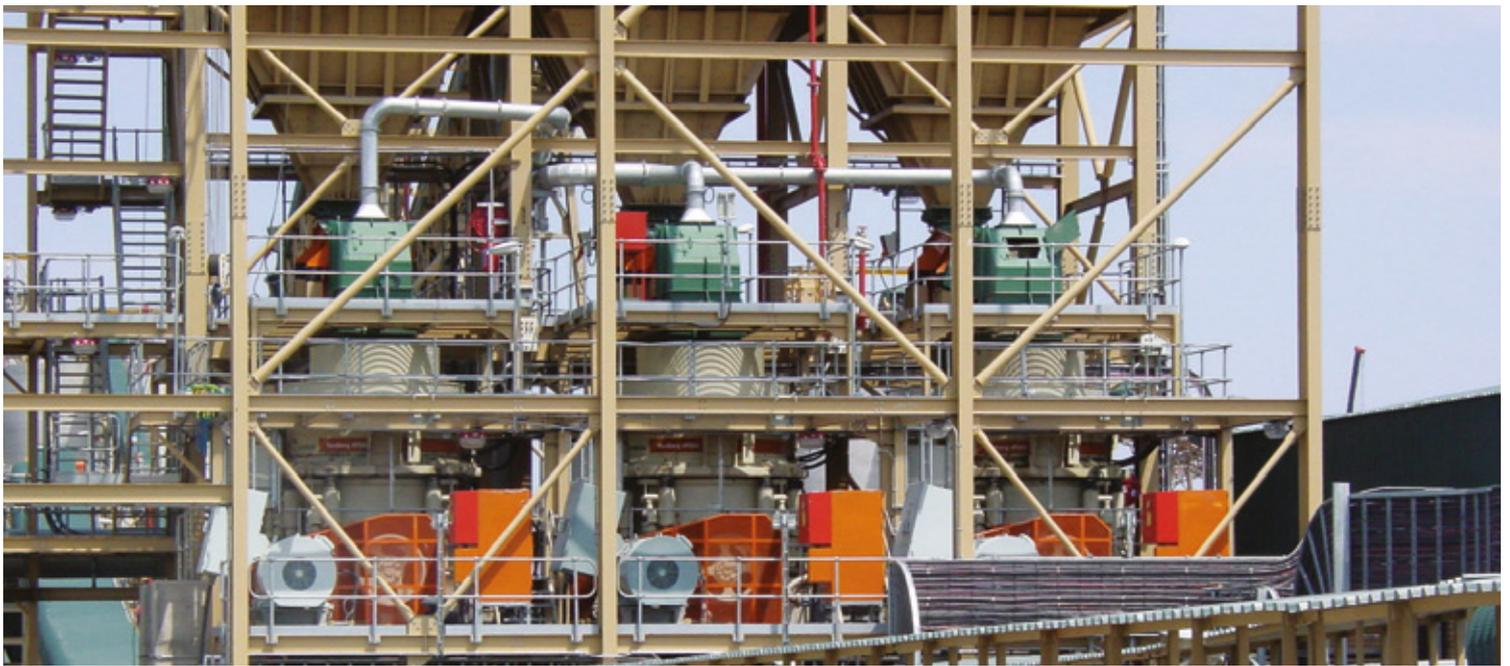
**4. Check the closed side setting. The setting should be close to the required product. The setting is too small if the adjustment ring is moving on the main frame (ring bounce).**
