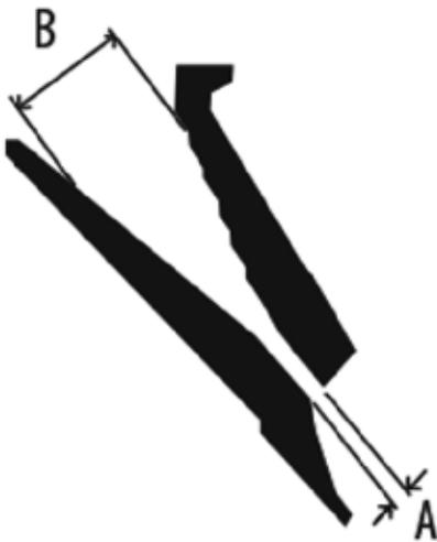
1. The minimum setting is that at which the crusher will operate without causing ring bounce. Depending on the crusher characteristics of the rock, this setting can change.
