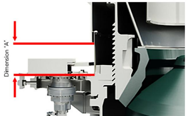
**Caution: A is given for a good wear. Meaning similar mantle and concave wear, without distorted wear profile = correct application according to cavity selected.**
