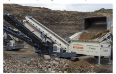
Large feed box allows closed circuit process.
