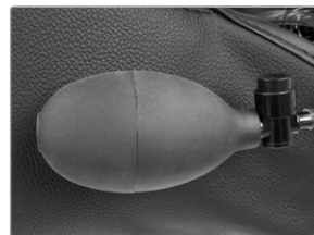
Air lumbar support To give good support to the lower back
