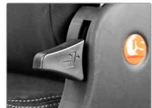
Backrest angle support 0 - 24° range to maximise user comfort
