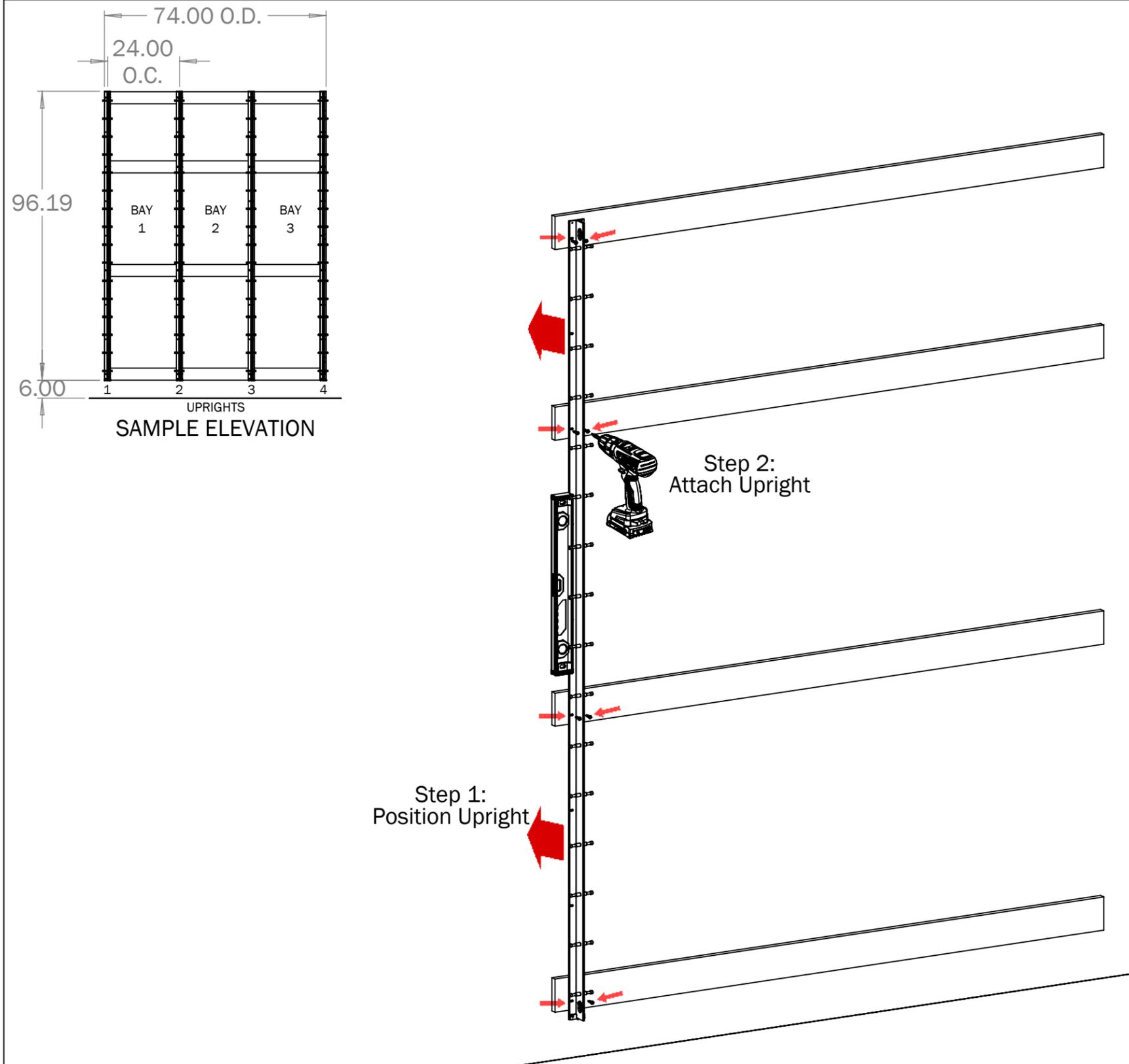
STEP 1: Hold the upright against the left side of the furring strips. The bottom left corner of the upright should align with the bottom left corner of the lowest furring strip.
