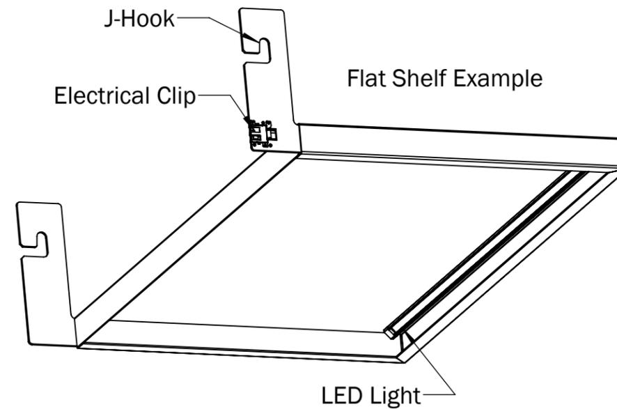
**GENERAL SCOPE:** System 1224 has a wide range of shelving and cabinet accessories, available in 24" and 48" wide, and many of those also come as electrified lit versions. Adding accessories is made effortless, utilizing the j-hook feature, and hanging from the upright pins. Install locations are vertically every 6" along the upright.
