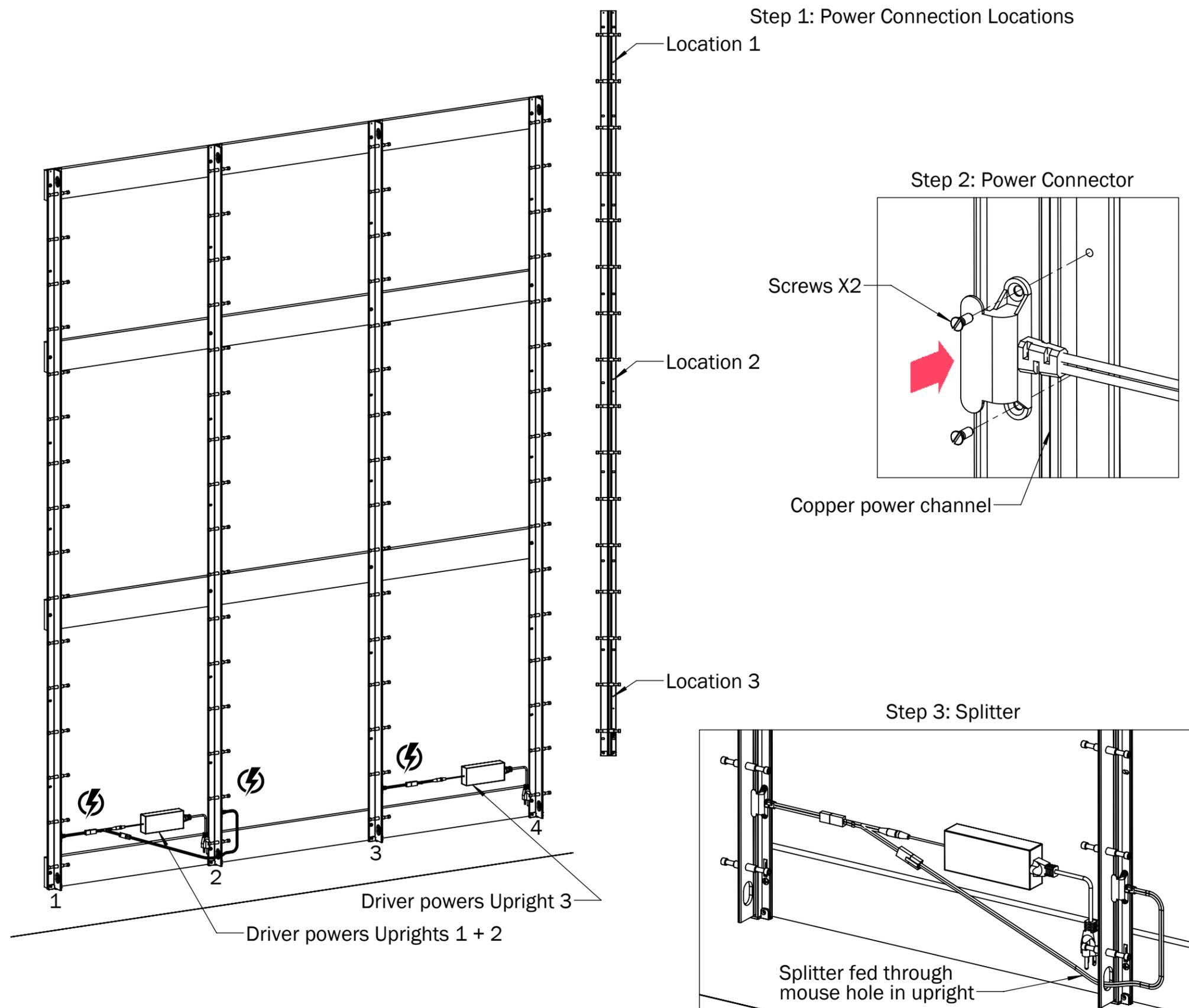
**General Scope:** The powering of the uprights is accomplished by using a driver connected to a power connector, which in turn is connected to the upright. The power connector makes contact with a copper channel that runs the length of the upright. The power needs of the setup will determine how many drivers are necessary to power the accessories. This example elevation will use a typical setup of one driver powering two uprights via a splitter.
