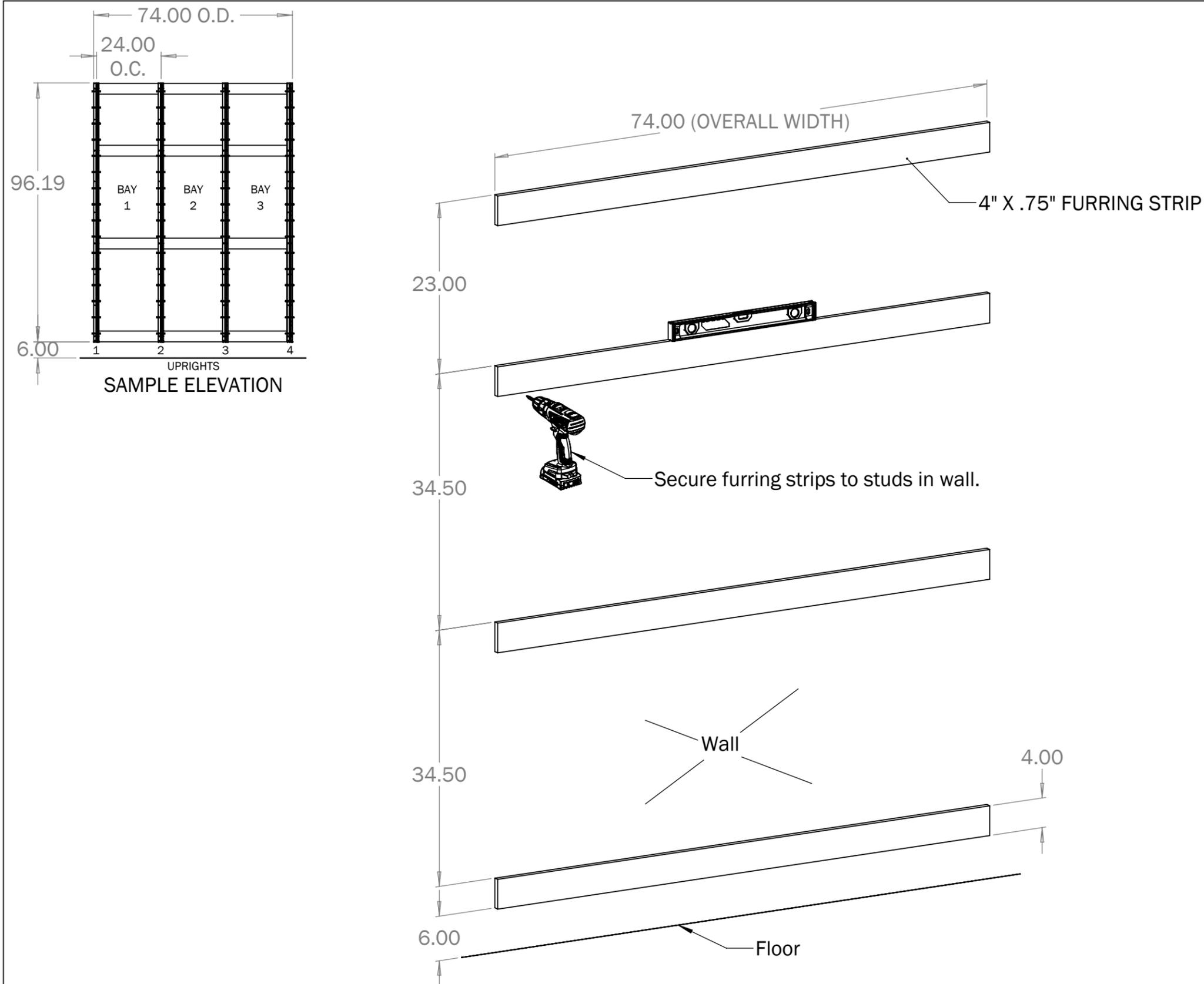
**BEFORE YOU BEGIN:** The following instructions will show a three bay elevation using typical 8' uprights as a sample installation. Although System 1224 can be secured directly to a suitable substrate wall, B+N recommends the use of furring strips. Furring strips will insure a strong and stable installation.
